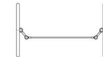
Tie rod mechanism Source: Mark Archibals, Design of Human-Powered Vehicles (2016)
