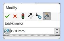
You are able to change Variables either by modifying their definition in the part itself (you can toggle between viewing the variable name or value withthe globe button) or through the feature tree like any other Solidworks Feature
